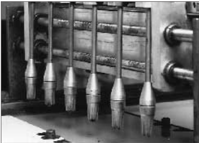
An installation used to blow away remnants of chocolate when filling
